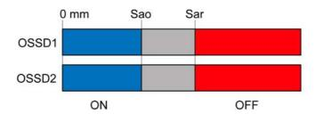
Guaranteed sensing distances for XCSR RFID Safety Switch are given in face to face configuration and without misalignment between the transponder and the reader:
