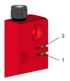
**LED 1** (TR) Transponder state **LED 2** (RD) Reader/Output state
