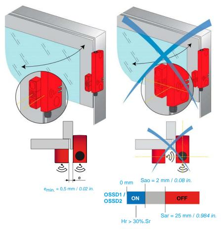
**e** Recommended minimum mounting distance between transponder and reader.
