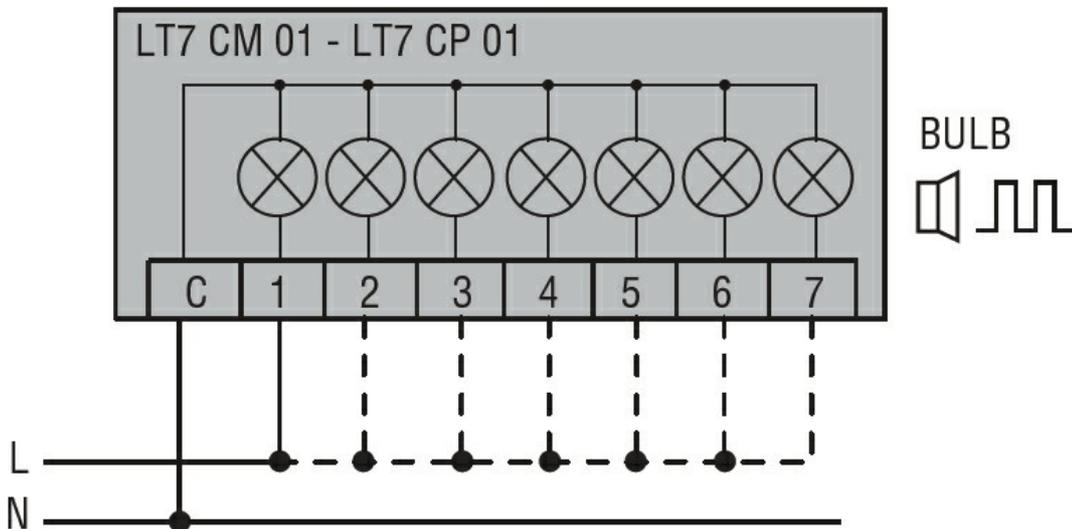
Connect terminals C and 1 as indicated to power the first module. If other modules are fitted, the respective terminals must be connected accordingly.
