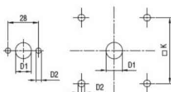
Drillings for 4 screws fixing
