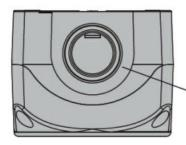
Knockout for M20/M25/PG13.5/PG16 (on top and bottom)
