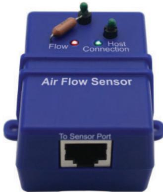
The airflow sensor is a switch type on/off style sensor. It is not a precision airflow measurement sensor, but rather an indicator of whether there is a presence or absence of airflow. A threshold can be set to determine the sensitivity of the sensor. Ideal for placing in-front of air intake or exhaust fans to indicate if the airflow is sufficient and as an early warning of failures in the cooling systems or fans.
