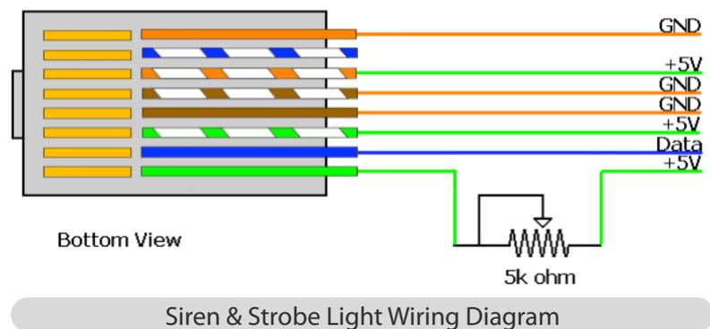
Alternatively, you can wire in a potentiometer, or a switch into the siren/strobe sensor. This would allow you to control the volume or disable the siren while leaving the strobe light active. You can wire in-line, a 5 ohm potentiometer (pot), or a switch with the siren, then it would be possible to adjust volume, or turn it on or off completely.
