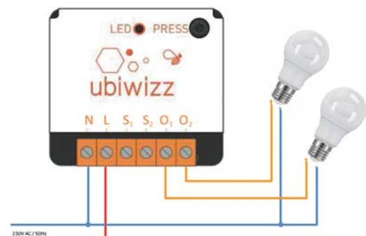
Câblage standard - Commande radio
