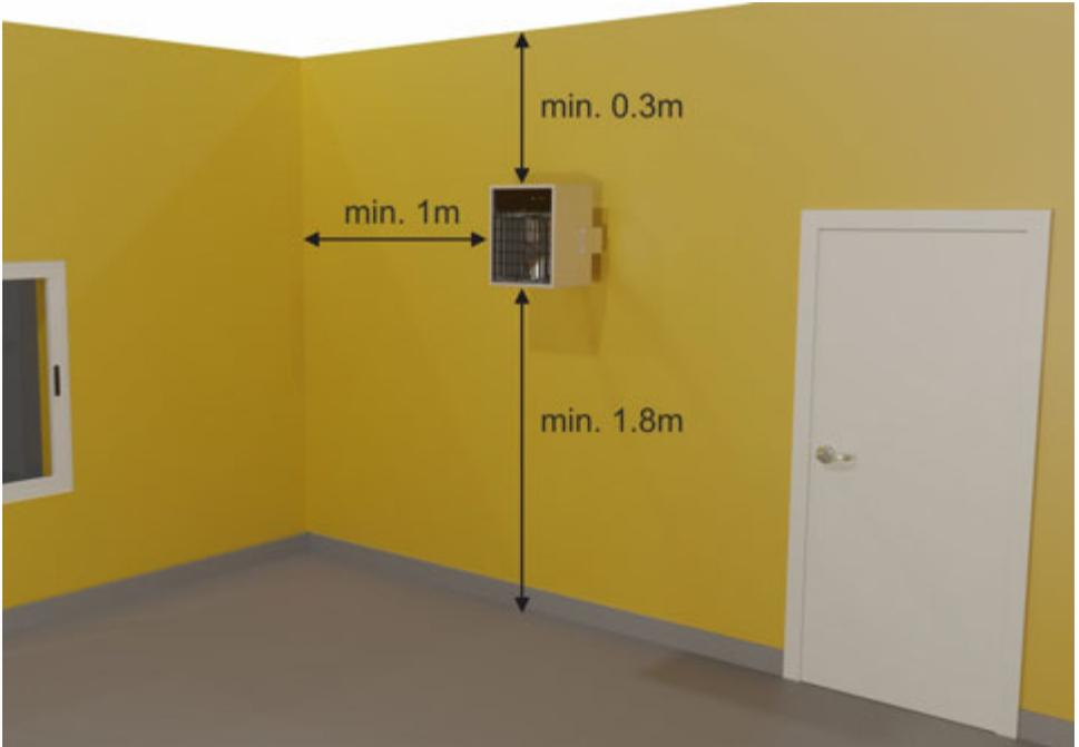
In order to ensure to the heater proper working conditions, the minimum distances from the ceiling, walls located on the sides of the heater and the minimum installation place height should be maintained.
