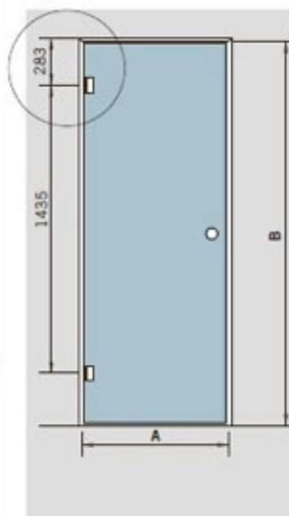
Example for measurements and set standard measurements for hinges and door levers.
