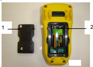
Figure 6: access to the battery
