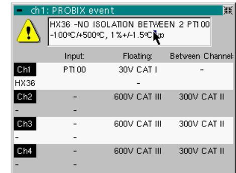
Measurements in «°C » are available 30 sec. after connection of HX0036 and a calibration phase.
