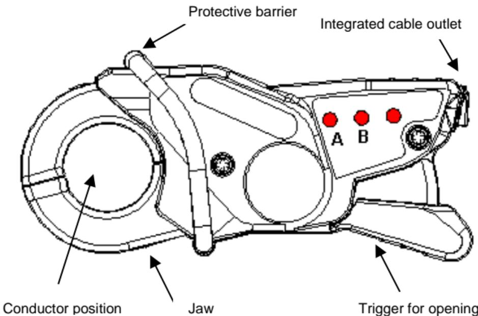
There are three pushbuttons on the side of the clamp:
