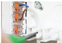
Insert the cable into the strain relief.
