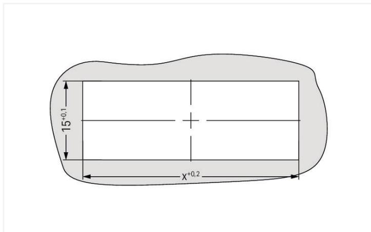
$X = (\text{pole no.} \times \text{pin spacing}) + 15.8 \text{ mm}$
