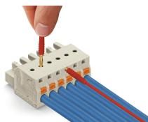
Testing parallel to conductor entry via integrated test ports – female connector with push-buttons and Push-in CAGE CLAMP® connection – touch contact perpendicular to conductor entry.
