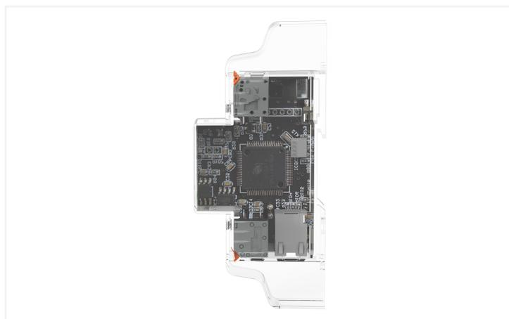
WAGO's communication module extends the WAGO Energy Meters and other Modbus RTU slaves with ETHERNET access. The Modbus TCP Module's design is based on the 879 Series Energy Meters and has the same profile as these. There are various options for connecting the communication module to the energy meters:
