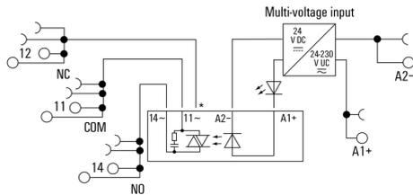
\*Contact is assembled in socket but not used with solid-state relays
