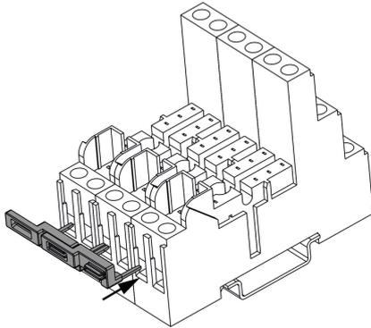
Plug the cross connection into wire-connection opening
