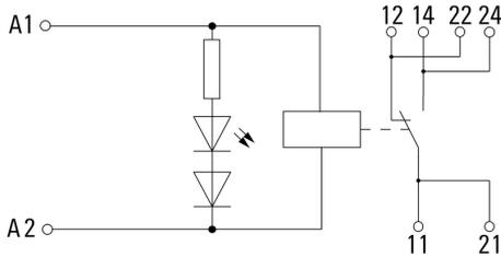
For full continuous current (16 A), the wire terminals 11 with 21, 12 with 22 and 14 with 24 must be bridged with a wire  $\geq 1,5 \text{ mm}^2$  at the socket.
