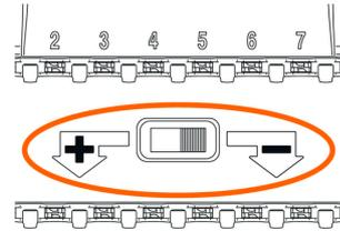
The potential switch, located between contact rows of TERMSERIES adapter, is used to switch the potential of the lower contact row to "+" or "-" potential of supply voltage.
