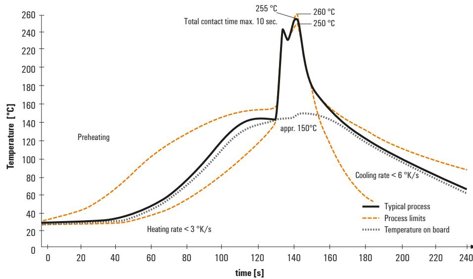
**Wave soldering profiles**
