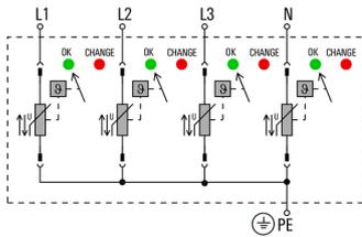
Schematic circuit diagram
