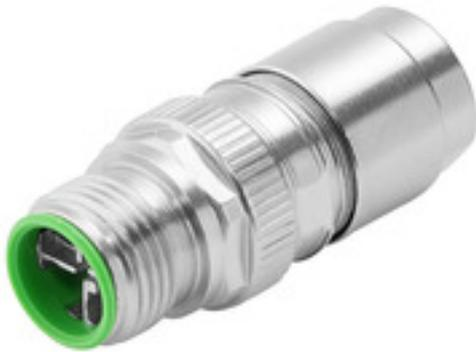
The 8pole M12 Mini crimp cable connector with X-coding and 90° cable exit is with compact dimensions and 8 cable exit positions predestined for difficult installation conditions. The cable clamp version with the wide cable clamp ranges from 4 up to 9 mm plus the fully shielded housing together with the shielded strain relief is the universal fail-safe solution for all common cables on the market.
